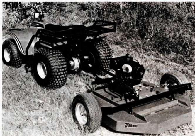
Self-contained mower cuts 36 in. swath.
