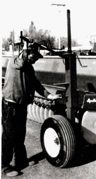
A hi-lift jack is used to raise and lower drills on transport.
