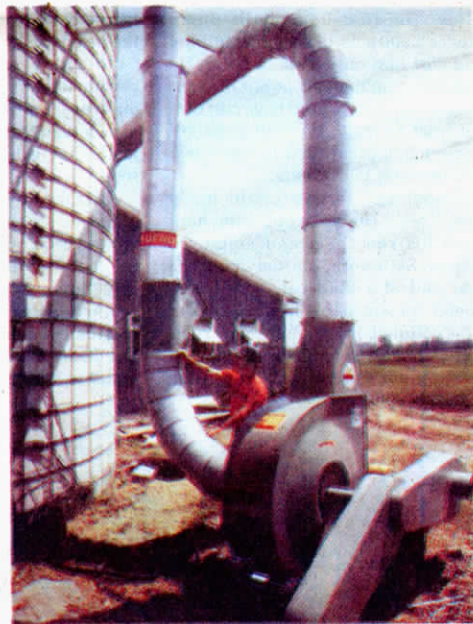
One Neuero pneumatic loading-unloading forage handling system serves two silos — a Harvestore and a Herd King — on the Nord and Jim Westover dairy farm, Clifton, Idaho.
