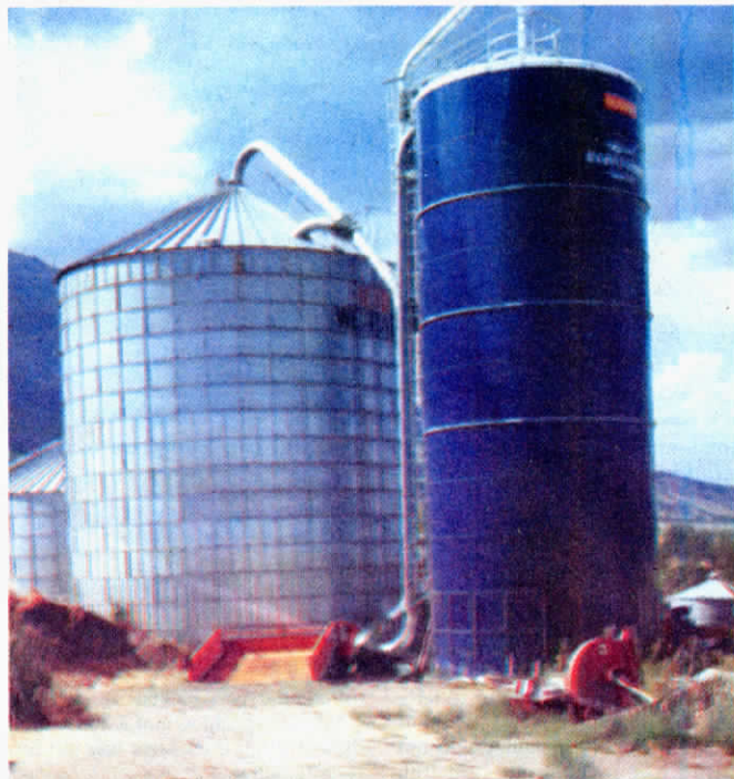
One Neuero pneumatic loading-unloading forage handling system serves two silos — a Harvestore and a Herd King — on the Nord and Jim Westover dairy farm, Clifton, Idaho.
