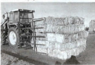
Company's 3-pt. mounted "squeeze transporter" can be used to haul up to 40 small bales at a time.
