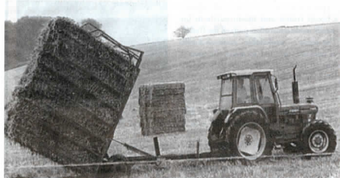
Bale transporter carries stacks to the barn or storage area and can be adjusted to carry either 56 or 72 small square bales at a time.
