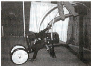
The 10-ft. wide drill hitch fits Cat. II and III quick hitches and can accommodate drills 10 to 14 ft. wide. You remove the drill's pull-type hitch and bolt the drill to new hitch.
