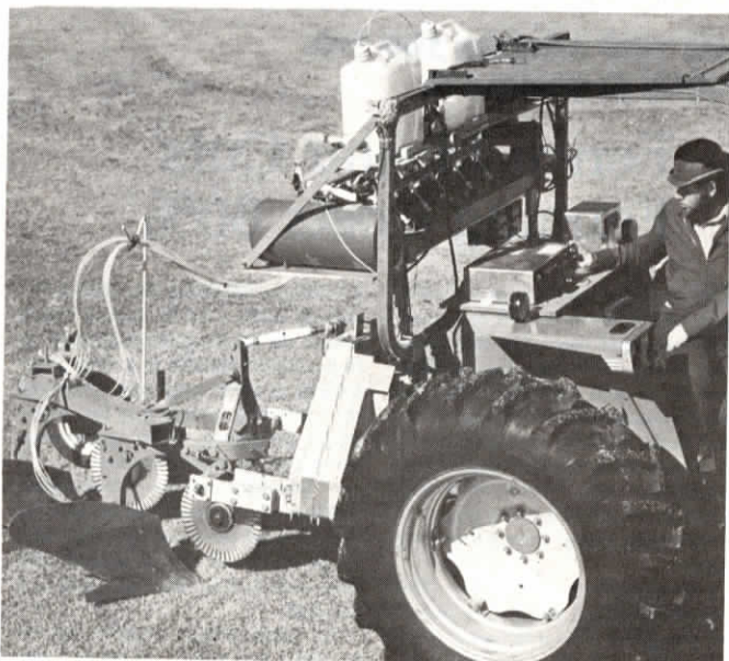
Grease "injector" designed for research tests at National Tillage Laboratory is more complicated than one a farmer might use. Lubricant being tested is completely water soluble and breaks down in the soil, leaving no residue.
