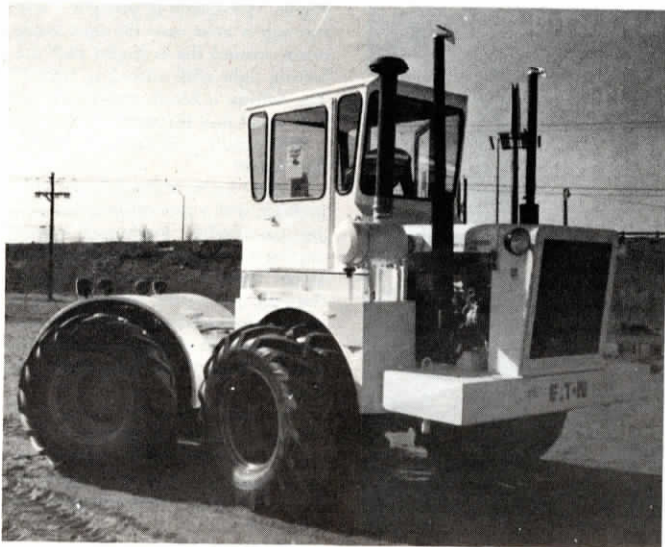
Klepper equipped this 1956 model Wagner tractor with a hydrostatic drive conversion kit. He retained only the original frame, axles and wheels.
