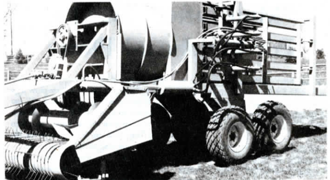
New machine makes 4 by 4 by 8-ft. bales using a new continuous compression process.
