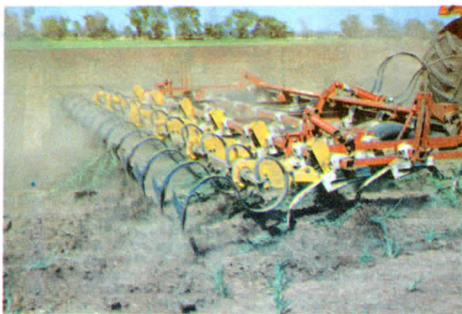
"Water Check" shovels move up and down 45 to 50 times per minute to form upwards of 12,000 water-holding "troughs" per acre.
