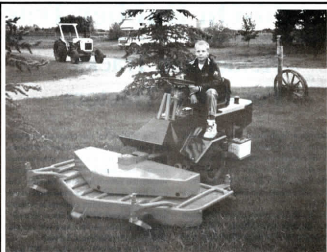
Schmidt used 1,200 cc engine from Datsun B210 car to power home-built mower.
