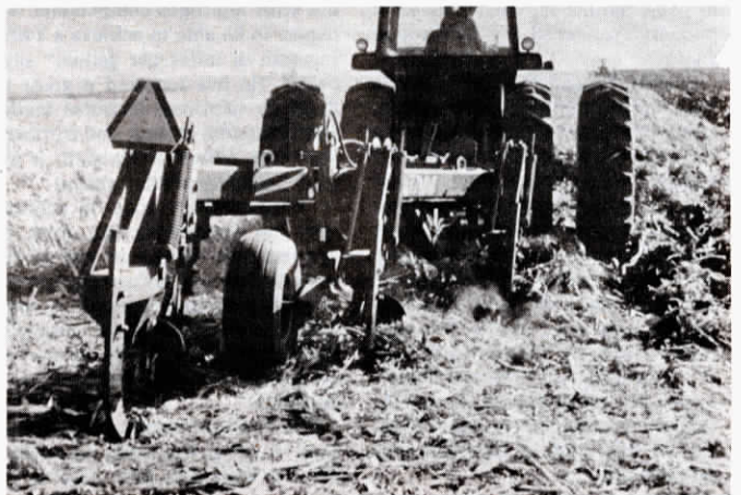
Compared to a conventional moldboard plow, every other bottom has been removed and a subsoil shank added behind each remaining bottom. Modified coverboards turn over just enough soil to cover the unplowed ground between the bottoms. Subsoil shanks then break up the soil under each of the shallow furrows.
