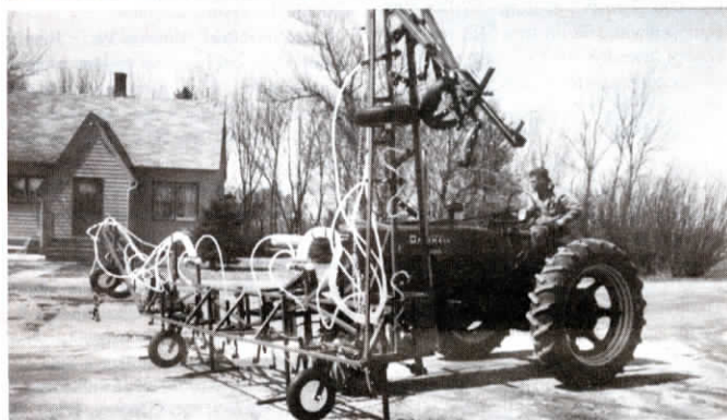
Boom extends 30 in. ahead of tractor and can be shifted 6 in. to either side on-the-go.
