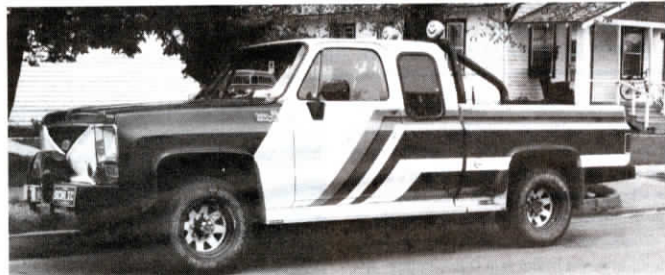
Extended cab is 21 in. longer than original cab and bed is 22 in. shorter.
