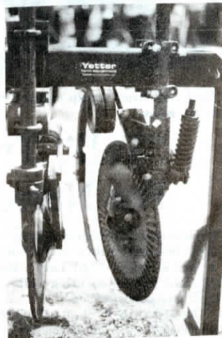
Up-front swivel lets narrow 1/4-in. wide shank and cutter swivel up to 30°.
