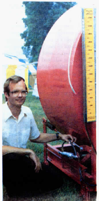
Feed load is tied into 2 by 6 in. cylinder which controls the scale's fluid level.
