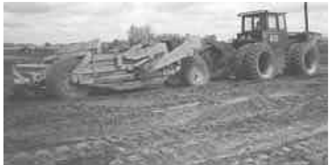
Rebuilt industrial scrapers were designed for use by highway building contractors.
