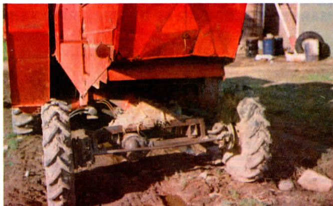
Sachar converted his 1965 International 315 combine to 4-WD by replacing rear steering axle with front axle off a 1/2-ton Chevrolet 4-WD pickup.
