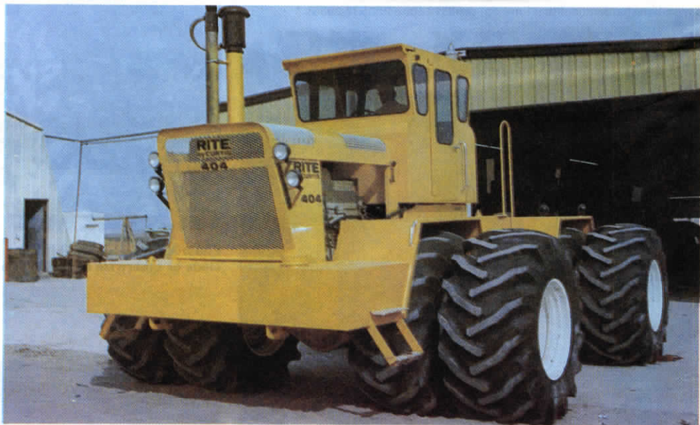
Outstanding feature of the new Rite tractors is the "clutchless" infinitely variable speed mechanical transmission. Model 404 boasts 400 hp. Other models ranging from 200 to 600 hp also available with the new-style transmission.
