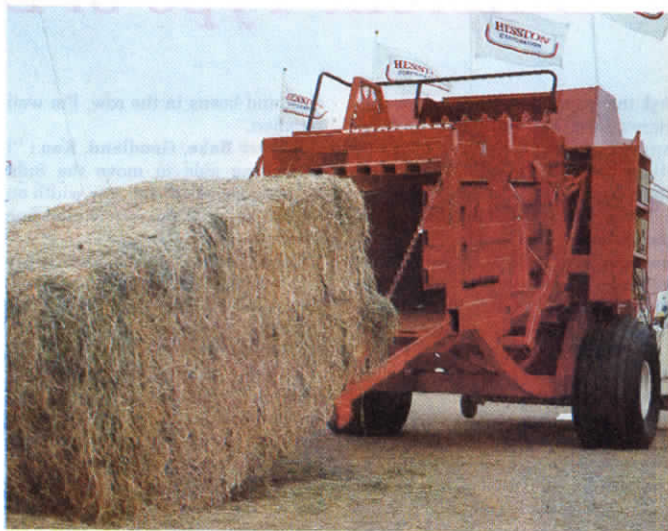
Individual rectangular bales made by the new Hesston prototype machine measure 46 in. wide, 50 in. high and 6 to 8 ft. long.
