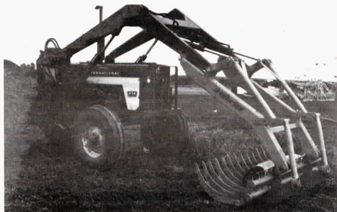
An optional fork, which mounts in place of the bucket, is "great for digging rocks out of fields or handling manure," according to the manufacturer.
