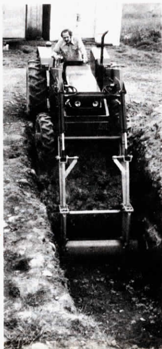
BenBucket digs straight-sided holes, trenches 7 ft. deep.
