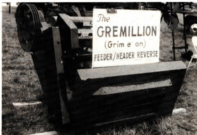
Reverser bolts to combine. Cleans out plug-ups by reversing feeder and header with a chain drive.
