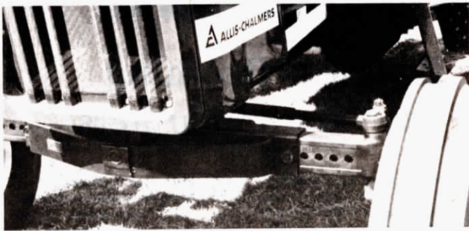
Kit extends wheelbase 10 in. on AC tractors, and up to 14 in. on Case tractors.
