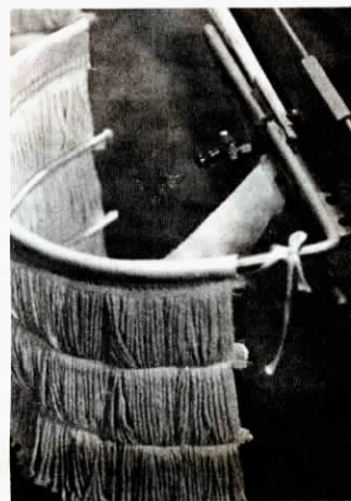
A drip strap beneath each nozzle "catches every drop."
