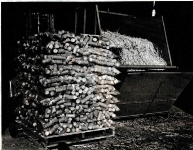
Big round bales of straw (in shredder) are converted into Strawloggs (2 in. dia. and 6 to 8 in. long) at the rate of up to 1,000 lbs. of processed "logs" per hour.
