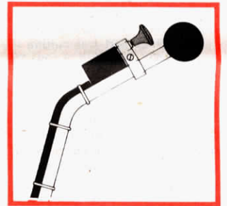
Electronic push-pull switch mounted on the floor shift lever.
