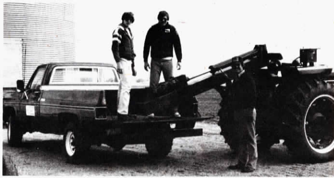
Huge splitter features a 40-ton ram cylinder with the wedge mounted on the ram rather than on the stop plate, as on most splitters.
