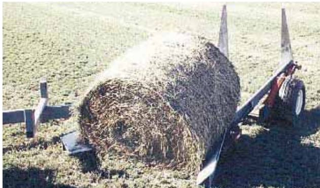
Front 5-ft. section of each rail spreads out to guide bales as they're being loaded. Slick plastic liners on bale arms help bales slide onto trailer.
