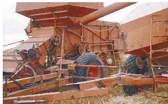
Unloading auger runs on drive pulleys on main shaft out of combine's gear box.
