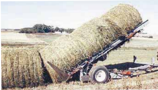
Simply designed, hydraulic bale hauler stacks bales one, two or three high.
