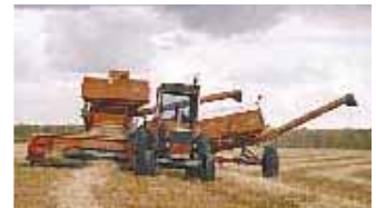
Combine and hopper pull evenly behind tractor. Hopper is angle-mounted to fit under auger.
