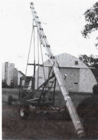
The Grain Hawk lowers under an 11-ft. door to move grain in or out of flat storage.
