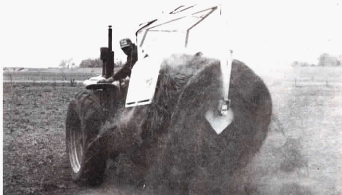
Hay Chief bale spike spins the bale, which is partially supported by a rear support arm.
