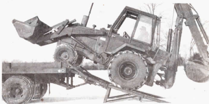
New ramp folds up flat, adding four extra feet to the truck bed.
