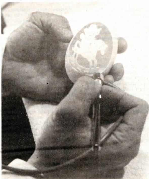
Spinks "engraves" turkey, goose and chicken egg shells with an air-powered drill that spins at 480,000 rpm's.
