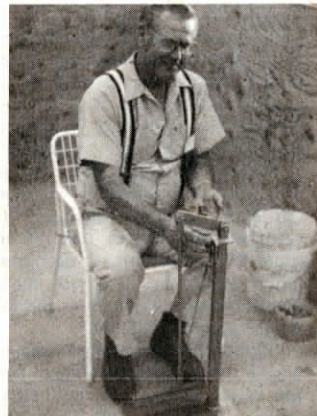
Lever cracks nuts against the head of a bolt.
