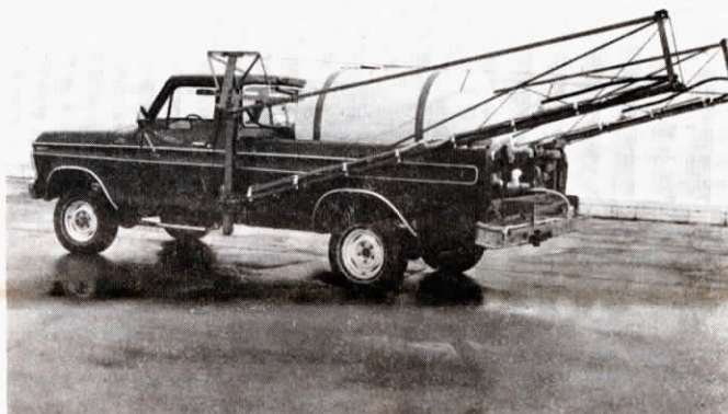
Spray booms are mounted in the center of the truck, behind cab.
