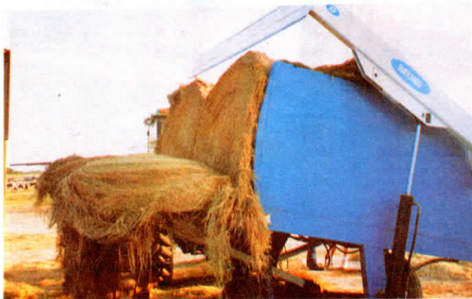
Bale slicer automatically cuts big bales into long-stemmed chunks using a hydraulic-powered guillotine-type knife.
