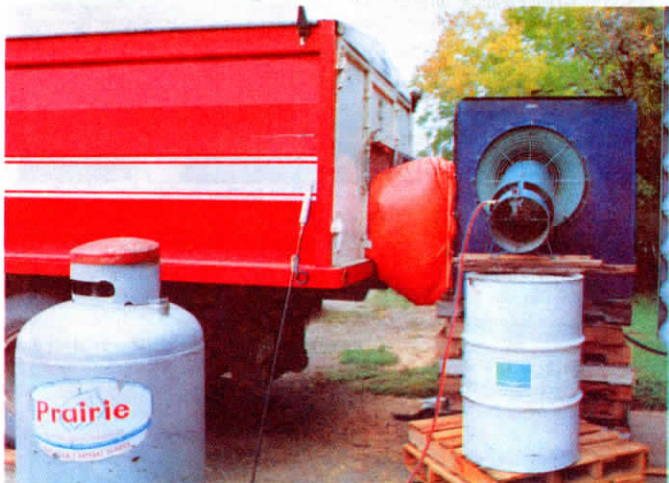
McNabb uses propane heater, fan, and inlet tube to dry grain in tandem-axle truck.
