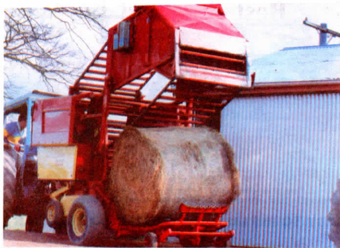
Bale is "kicked" onto pipe frame directly behind baler tailgate.
