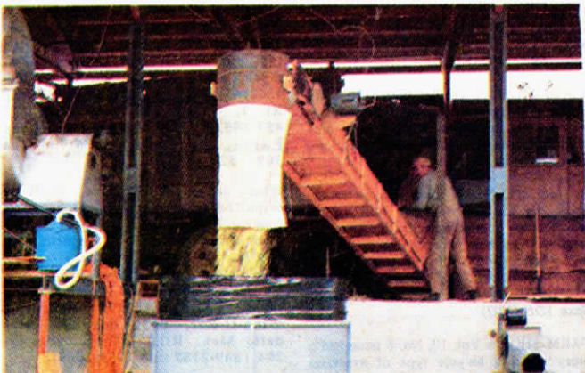
One person feeds conveyor and another walks on material inside of bag to pack it down.
