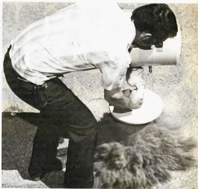
Pressing handle on Air Blaster tank sends even blast of air through entire filter to remove dirt.
