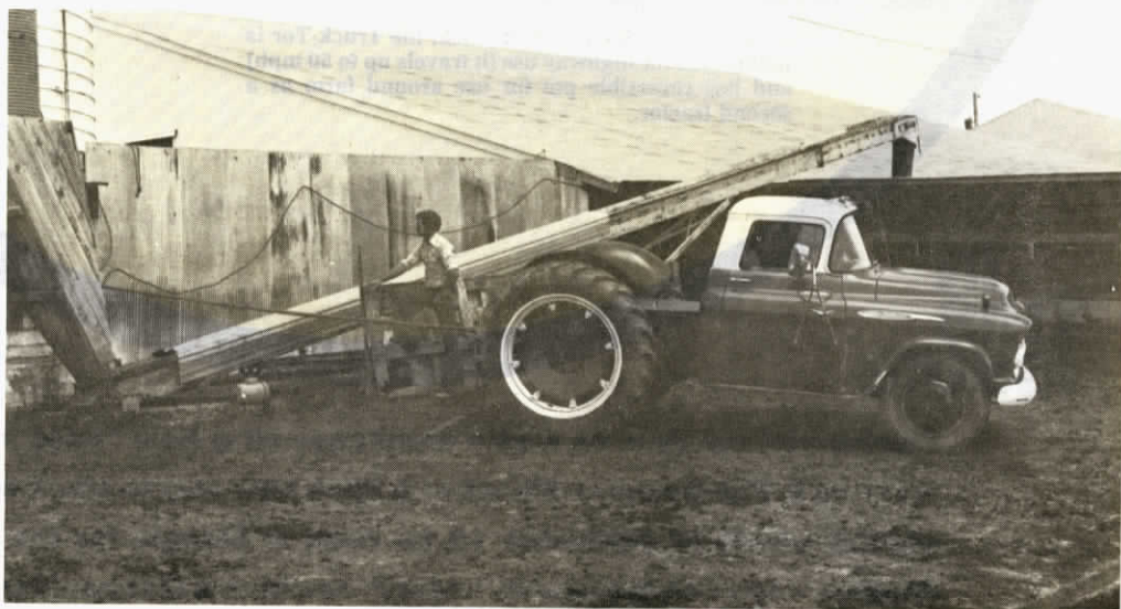
Steve Boendor says his Truck-Tor's reversible pto is handy for lowering, raising his silo unloader.
