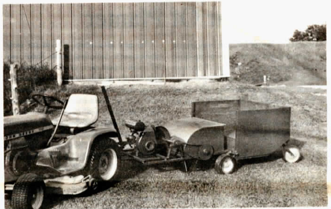
The sweeper's 24-in. dia. nylon brush is driven by a 1 1/2 hp. gas engine.
