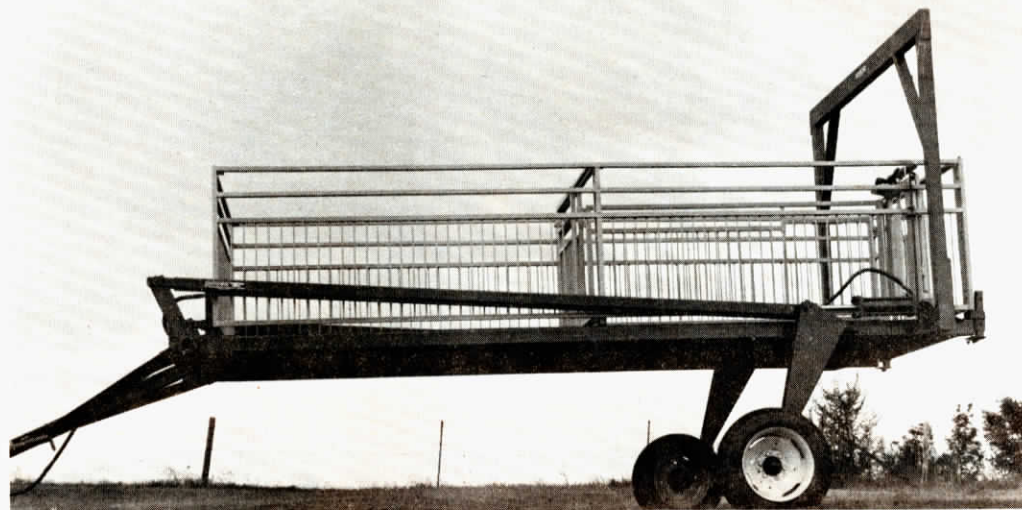
Roose hydraulic trailer can be used to haul livestock, big round bales, machinery and anything else that will fit on a flatbed. Converts to a round bale mover by removing six bolts and lowering pen and flatbed to the ground.
