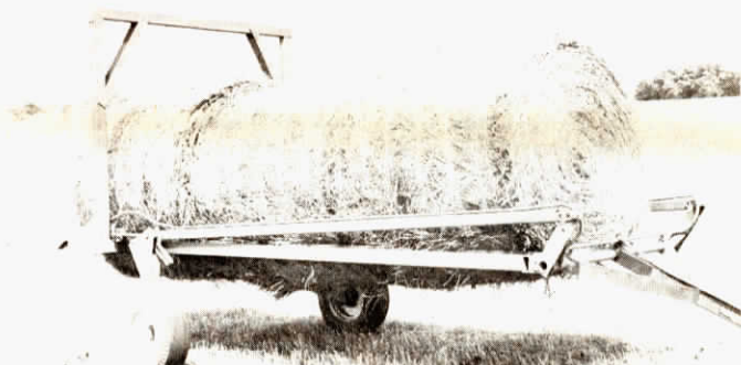
Three-bale model has high 50 in. clearance for moving over ditches and muddy lots. A four bale model with 40 in. clearance also available.
