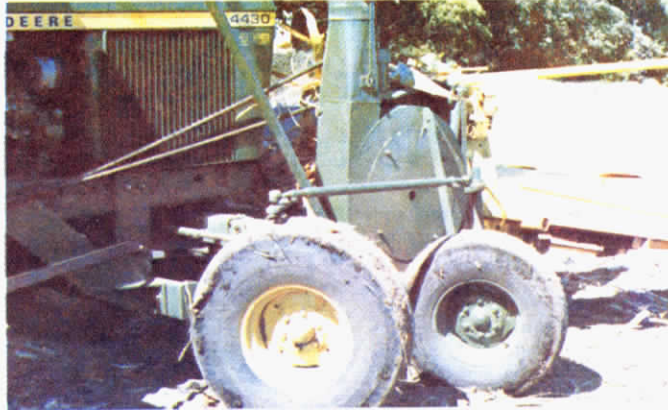
Converted front-hitched chopper rides on a special dolly. Wheels of the "Chopper Dolly" steer in exact sync with front tractor wheels.
