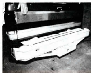
"Bale Bumper" folds into attractive bumper when not in use.
