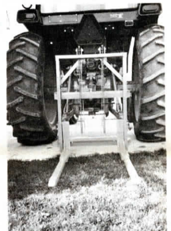
Pair of roller chains, anchored to drawbar and threaded through a pair of sprockets at top of frame, double lifting height of standard 3-pt.
