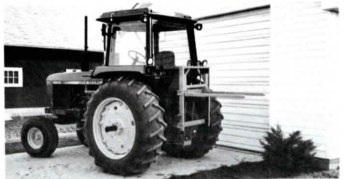
"The $265 fork raises to 5 ft. and does the work of forklifts costing $2,000 or more," says manufacturer.
