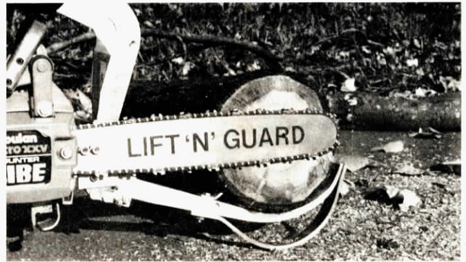
Lightweight Lift 'N' Guard slips under log automatically as you cut, so there's no pinching or dulling of saw chain.
