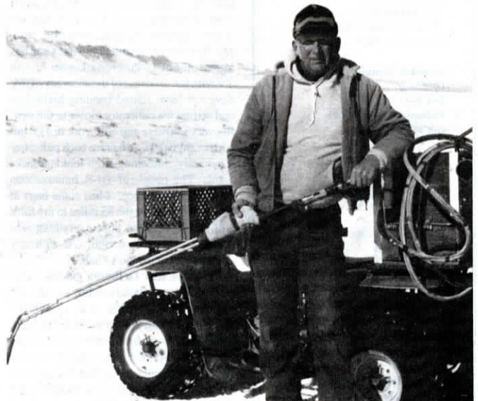
New gopher blaster pumps oxygen and propane down into tunnels and sets off an explosion with a spark plug mounted at the tip of the wand, killing an average of 4 to 5 gophers per blast.
