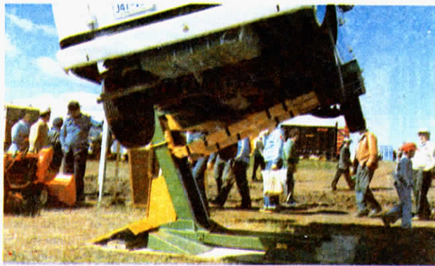
Wonder Hoist can either lift load horizontally, or with a 25° tilt. When at top of lift, outer edge of vehicle will be 6 ft. above ground. Lifts up to 6,500 lbs.
