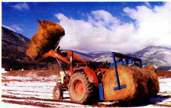
Two-bale model picks up 2 side-by-side bales. Loader-mounted bale fork grabs two bales at once.
