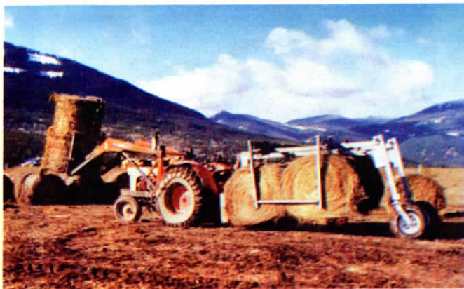
Four-bale model picks up 4 bales sitting side by side. To load bales, rear support wheels raise up hydraulically so you can back over bales, using 3-pt. to hold rig up.
