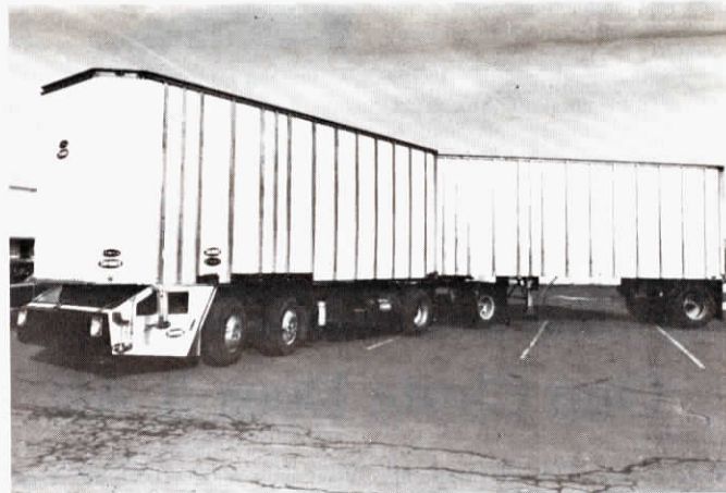
Low-slung cab, tucked under truck box, provides driver with good visibility ahead and to sides, says manufacturer.
