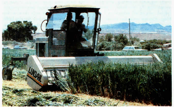
Hay is cut by cutting teeth welded to outside edge of lower auger, and conditioned by larger upper auger before exiting the back into side-side windrows.
