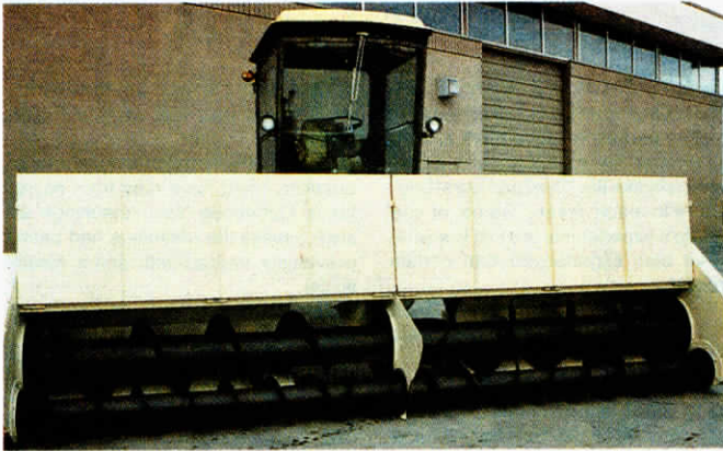
Mounted on a self-propelled swather chassis, new mower easily cuts through tall, twisted or tangled hay, says manufacturer.
