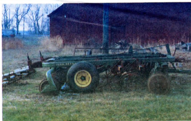
Stadler's home-built tillage tool has a row of discs up front, field cultivator shanks in the middle and packer rollers at the back. A 3-section harrow trails behind.
