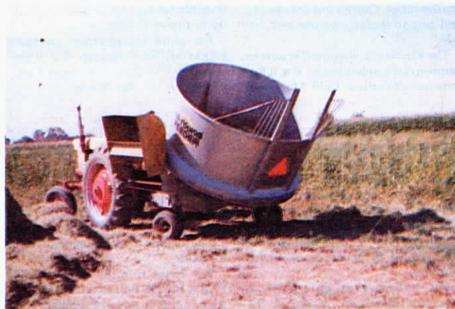
Entire tub tilts to ground to pick up bales via the twin forks mounted on side of the tub.
