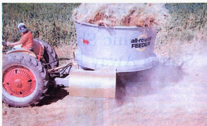
The All-Around Feeder for big bales isn't a grinder. Chopping is done by swinging flails.
