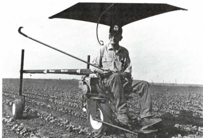
John Weber's "Weber Weeder" allows one man to weed six 30 in. rows right from the driver's seat. Optional box can be used to carry water, chemical equipment for spot spraying, fencing tools, and so forth.
