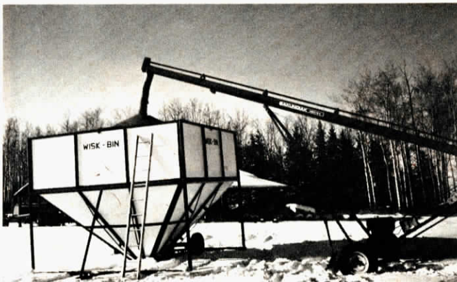
The bottom of the bin rests directly on the ground when stationary, supporting the major part of the weight. It rides on two wheels for transport.
