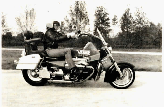
Custom-built bike sports a Buick V-8 engine. Strickland built his own transmission and driveline from the ground up.
