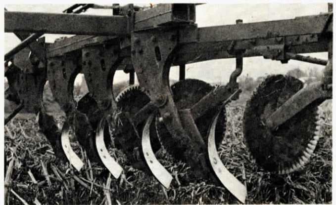
Reversible 4-in. wide chisel boards bolt directly to moldboard plow shanks.
