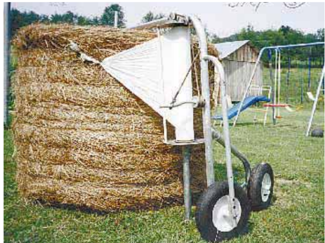
Two-wheeled unit carries a 30-in. wide roll of plastic and has an arm with a short spear that sticks into top center of bale. You roll unit around bale, using a hand-cranked winch to move the roll of plastic down.
