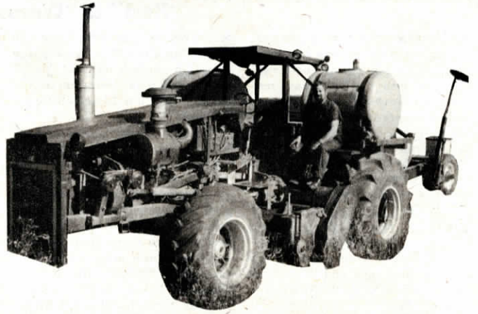
International planter mounts at rear of big rig. A spray boom applies herbicides just ahead of the rototiller.
