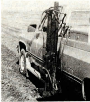
Rig takes a 10-in. long core sample from frozen ground in 25 sec.
