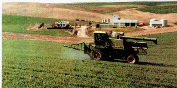
Wigen mounts a 600 gal. spray tank in the grain hopper and adds an 80 ft. boom, then converts back for harvest.
