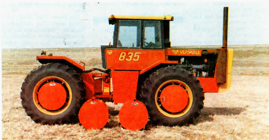
To add weight to tractor, fill tanks with water. Pull two plugs and extra weight drains away.
