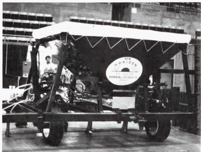
Seven over-sized injection knives inject fertilizer and ammonia at depths of 6 to 14 in.
