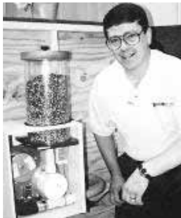
Bob Tessier's feeder refills with seed from your house or garage using a computer-controlled air delivery system.
