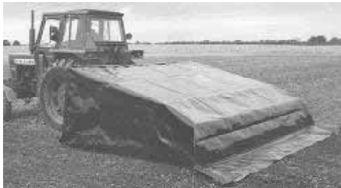
Covering tillage tools with a shroud simulates nighttime work, say researchers.
