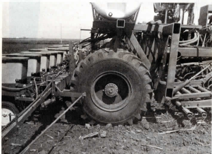
Power to hydraulic motors in all 12 wheels on the Culti-Planter is supplied by a 320 hp diesel engine which powers two hydraulic pumps. Goodyear Terra tires used on Crow's Culti-Packer measure 48 by 20.00 by 20.
