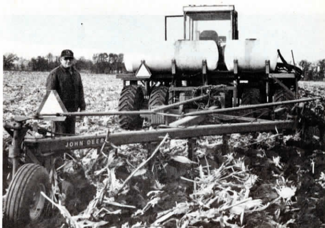
For plowing, the rig is reduced from 12 to 6 drive wheels. The 15 ft. wide power unit easily handles a seven bottom 18 in. plow. Note that cab, not shown in photo on left, has been added.
