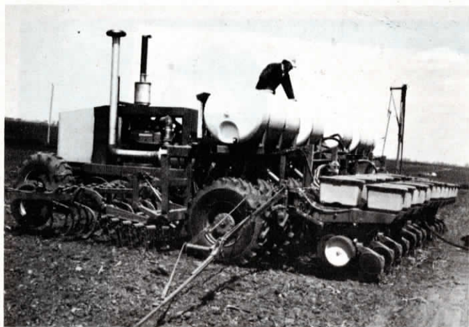
Culti-Planter "floats" on 12 drive wheels. A planter unit directly behind each flotation Terra Tire plants in the seedbed firmed up by the tire for nearly perfect stands.
