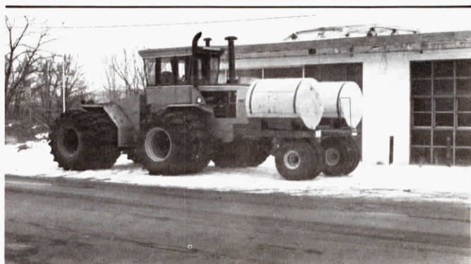
Wheels on the front-mounted Jim Dandy carriage are "free swinging" and don't interfere with driving. It carries tanks low enough so as not to interfere with driver's vision.
