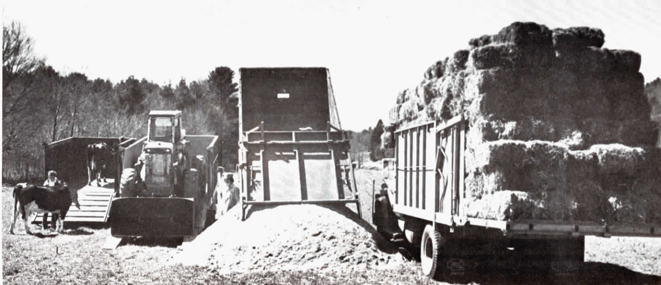
All-purpose gate swings up from top for dumping, lays out flat for an extension bed (for hauling bales, for example), and drops down to serve as a ramp for loading cattle, tractors or other equipment.
