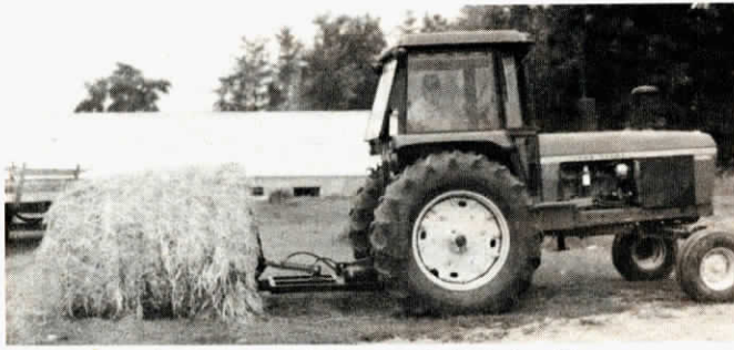
Baler carrier folds to ground for easy big bale handling.
