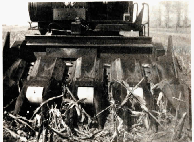
Each row unit features two snouts with a rotating cylinder, equipped with retractable fingers, in between.
